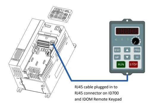
The Following set up will allow the IDOM Remote Keypad to control the ID700 – Start/Stop & Speed control via the potentiometer.
